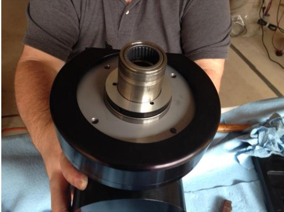
Photo 4. Gear housing fitted. Make sure that during installation you do not bump the gears.
