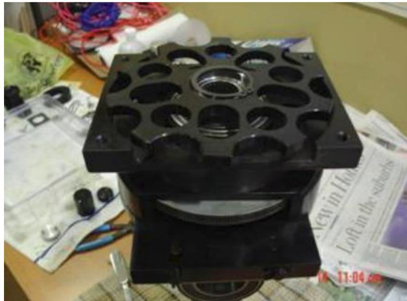
Photo 11. Snap ring shown before the pressure wheel is screwed down to permit installation. Photo from Titan Tips.
