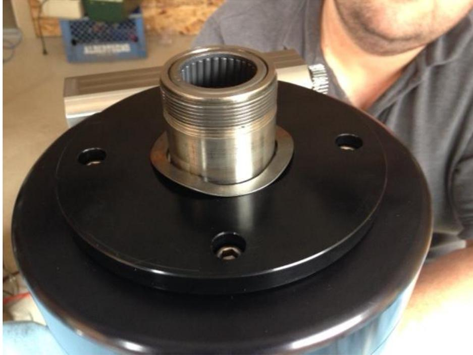
Photo 6. This is the first part of the installation that differs from Titan Tips. Compare to photos 8 and 9 below. The wavy washer is installed in the machined recess of the lower clutch plate BEFORE the installation of the clutch pad (see Photo 7).
