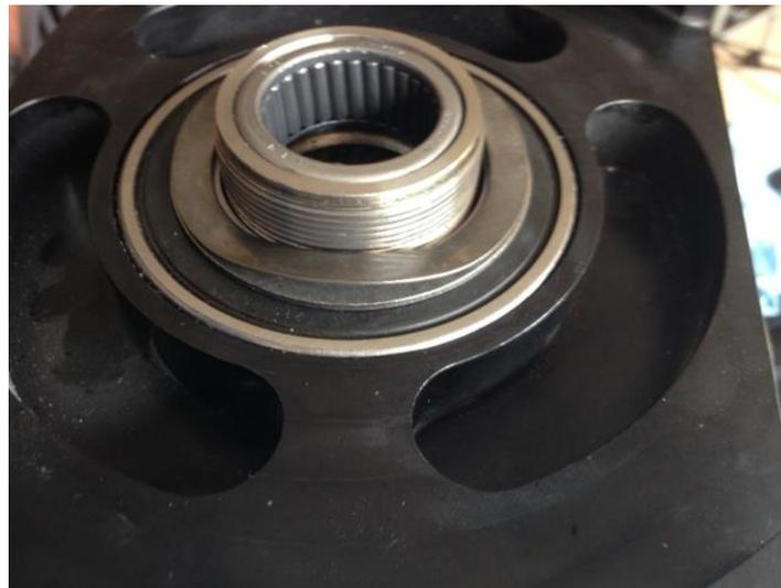
Photo 9. Detail of Photo 8. Again, ONLY the flat washer is installed, NOT the wavy washer and not two wavy washers. More explanation: If you try to install as in this photo, the pressure wheel does not work properly, it binds because there is not enough clearance once the snap ring is installed.
